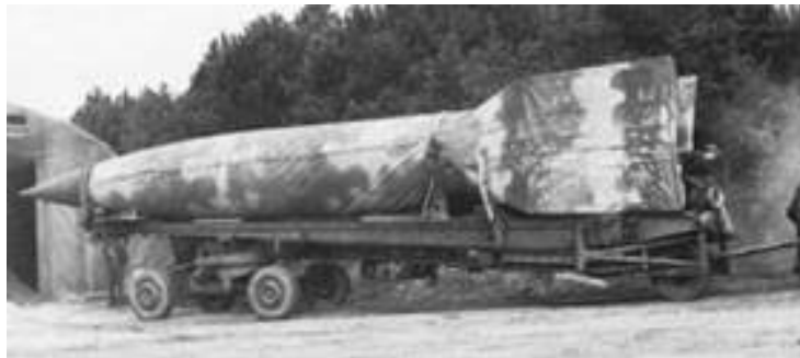
A V2 rocket on the Meillerwagen. The ragged edge colour pattern indicates it is one of the rockets during its operational phase. The Meillerwagen was used to transport the V2 to the firing site and used to raise the rocket
