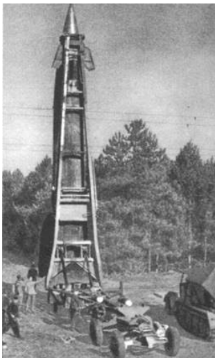
A V2 rocket on the Meillerwagen. The ragged edge colour pattern indicates it is one of the rockets during its operational phase. The Meillerwagen was used to transport the V2 to the firing site and used to raise the rocket
