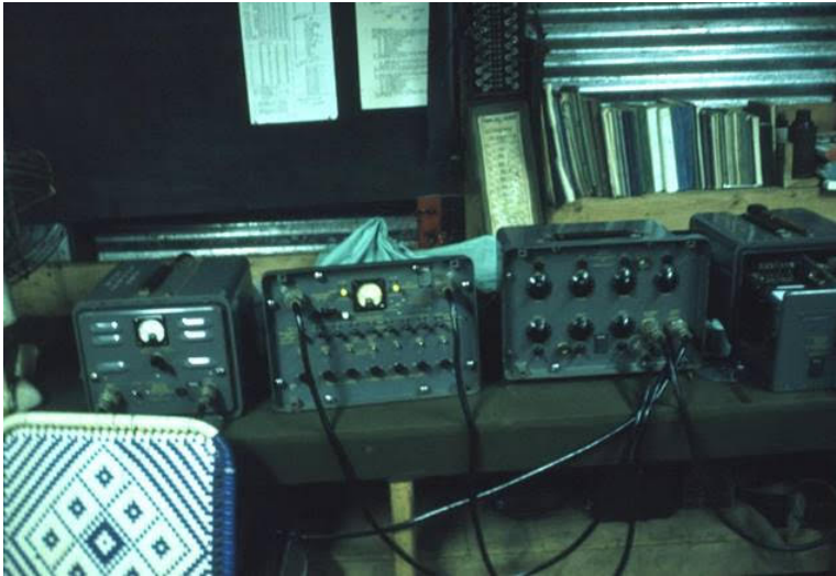
No 5 Sound ranging Equipment - Power Supply, Lines Test Unit, Amplifier, Recorder
