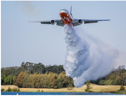
The DC-10 Very Large Airtanker, nicknamed Southern Belle, holds almost 44,000 litres of water, which it can drop at the speed of 280km/h
