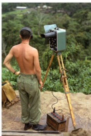
Lt. Ian Yerbury operating Tellurometer on survey operation Nui Dat. 1967
