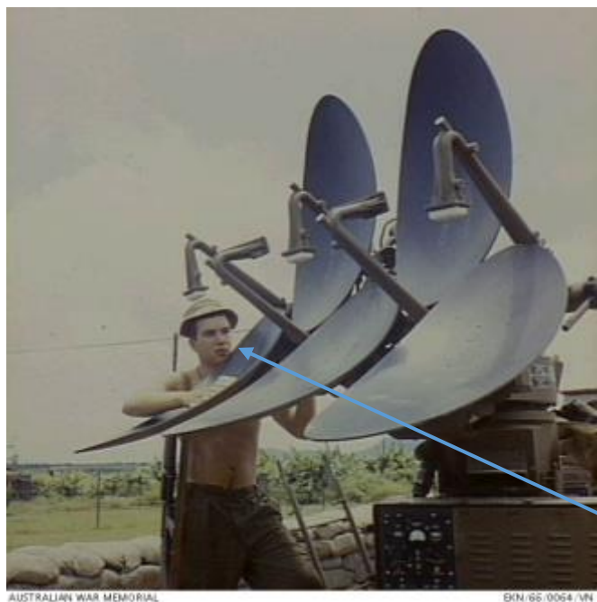
Nui Dat, South Vietnam. 1966. Radar equipment for locating and detecting enemy artillery positions, used by 131 st Divisional Locating Battery, Royal Australian Artillery, 1 st Australian Task Force (1ATF).
