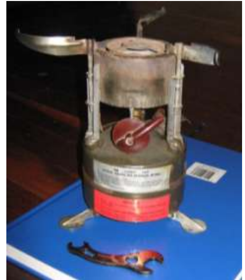
Stove, Gasoline Burner, M1950 - Personal Stove
