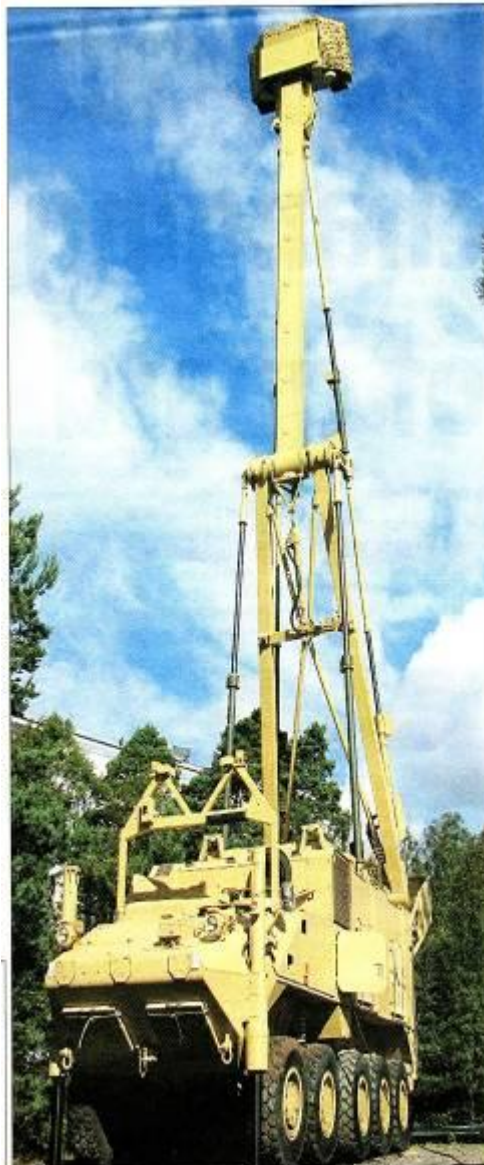
Impressive: The giraffe agile multi beam 740 radar system in extended mode. New counter-rocket and mortar capabilities are bound for Afghanistan.
